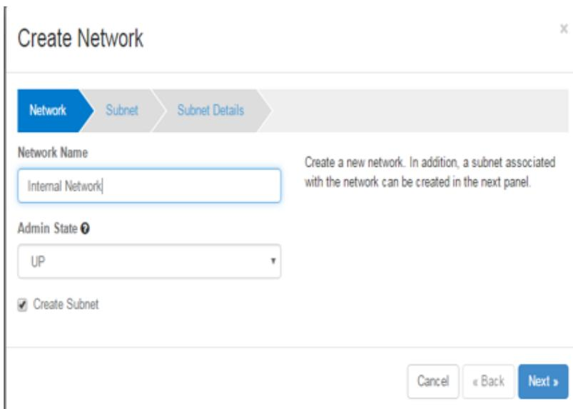
The screenshot shows the 'Create Network' wizard. It has a progress bar with three steps: 'Network' (active), 'Subnet', and 'Subnet Details'. The form includes the following fields and options:
